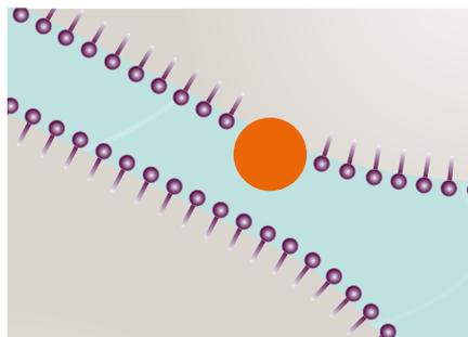
Entering of defoamer oil droplet in air/water interface
