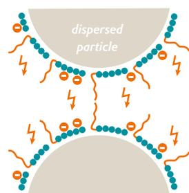
The main function is to break up the active material agglomeration and prevent flocculation during formulation (slurry mixing).
