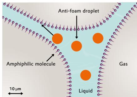
Defoamer oil droplet in foam lamella, stabilized by surfactants
