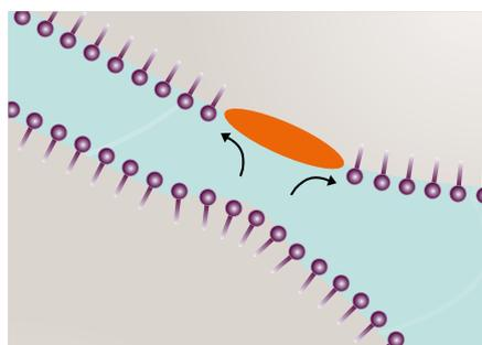
Spreading of defoamer oil droplet on air/water interface
